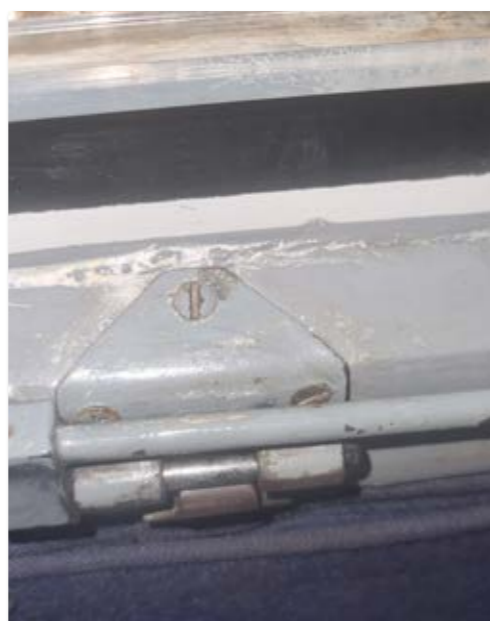
ABOVE: Figure 3, latch appears locked, but is NOT pushed through the sleeve on the fuselage frame.
