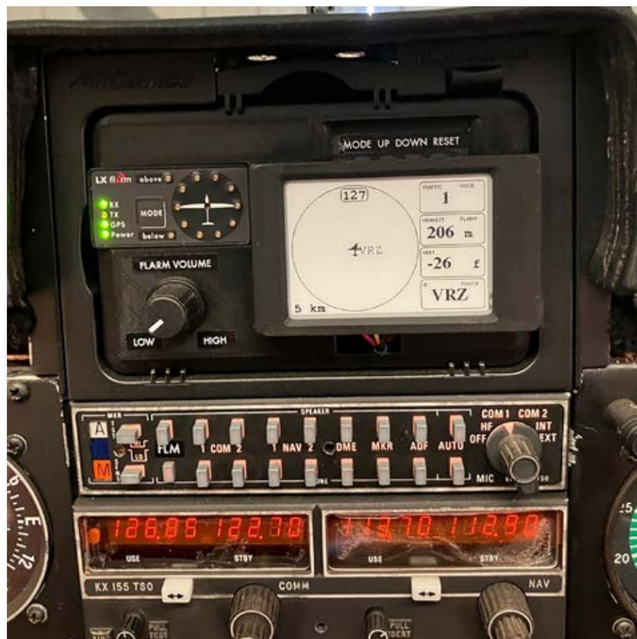
BELOW: WAGA SkyView installed in a Maul tug with voice alerts to pilot headset via the comms panel.
