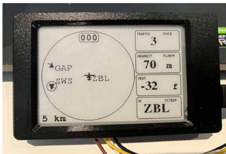
ABOVE: Radar View showing three aircraft in proximity. The host aircraft is a tug with ZBL on tow. SWS is another tug that has just released glider GAP
