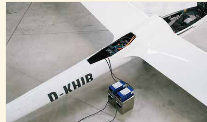
The LS8-e Neo with an FES installed. The photographs show the propeller extended (ABOVE) and the engine bay with battery pack (BELOW).
