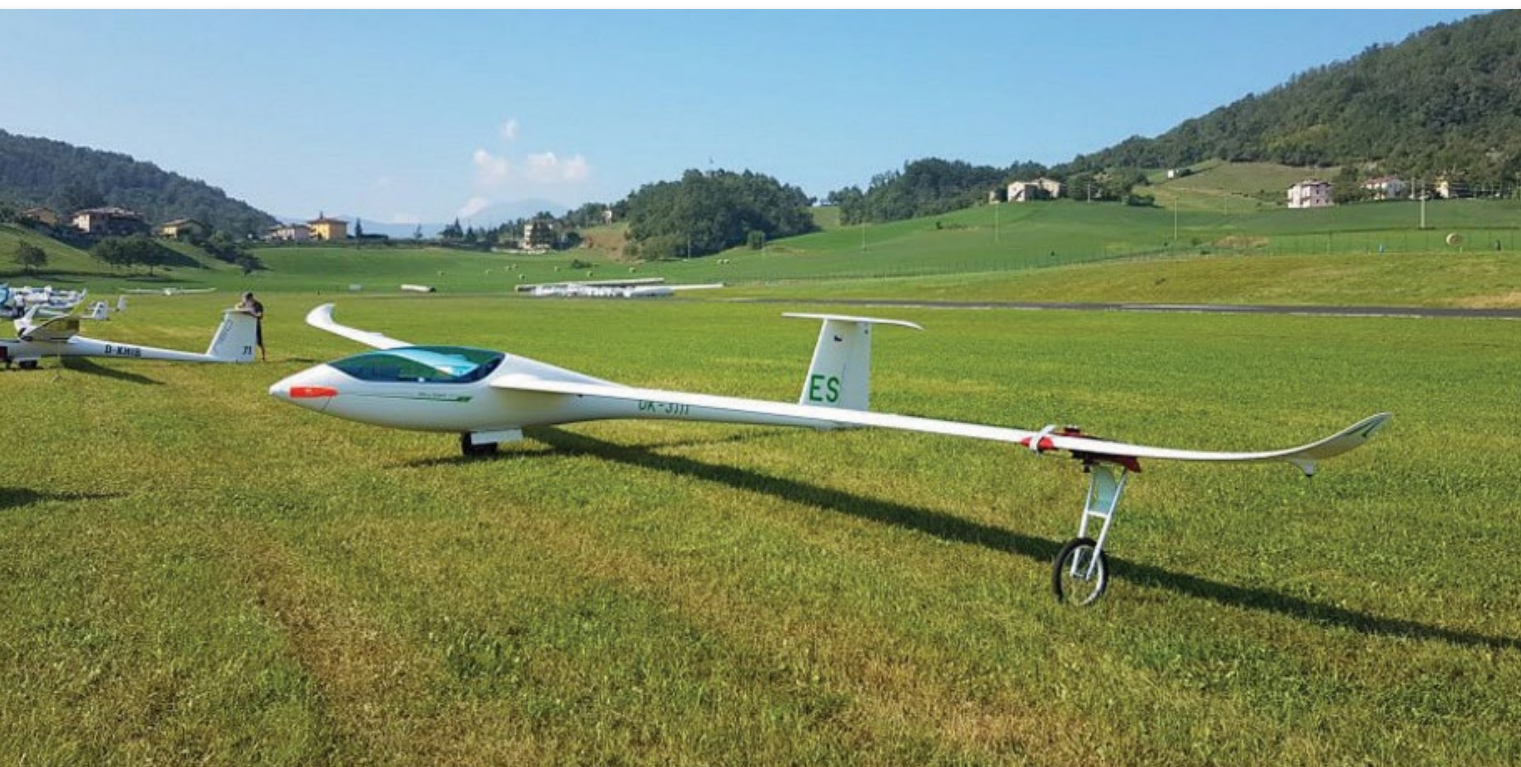
ABOVE: The Hph 304 ES that Markus flew with its orange FES propeller blades closed against the fuselage.
