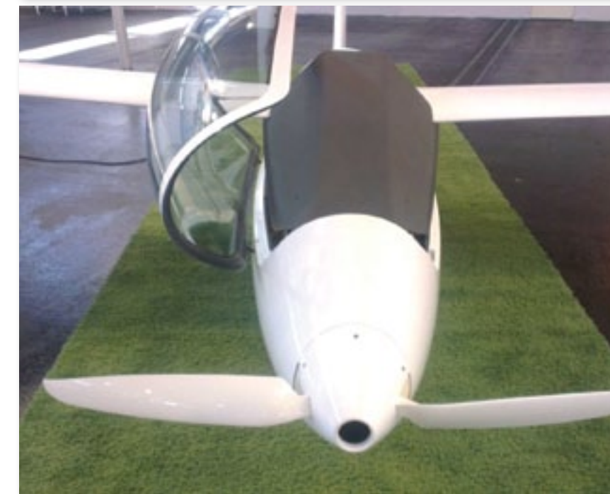
TOP : Propeller closed and flush on the fuselage
