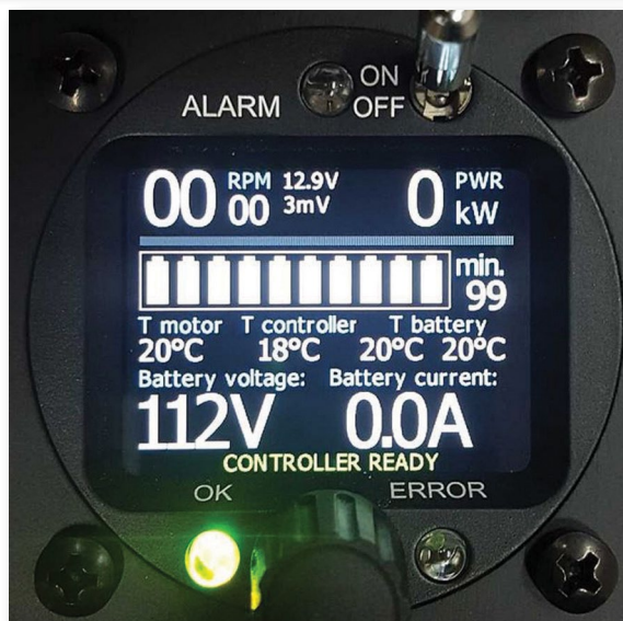
ABOVE: FCU – FES Control Unit Here are some rough numbers - Maximum power: max power 23 kW (30 hp), at 4500 RPM Continuous power: 16kW continuous power at 116V Max motor RPM: 4500 RPM Recommended RPM: 3000 RPM for horizontal flight; Climb - 1200 m (3900 ft) for the 18m class sailplanes at 450kg take-off weight (without water ballast); LAK17B FES, Ventus 2cxa FES, Discus 2c FES, HPH 304ES
