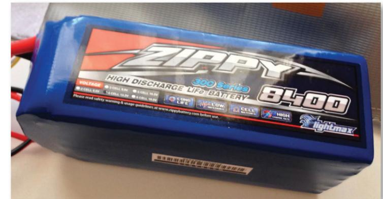
28.4AH. At current consumptions as per table 1, that is close to 28 hours of continuous flying, enough to run the entire flight deck very comfortably plus the ability charge phones, run cameras, have future ADS-B Out technologies and even put in toe warmers for wave flying!
