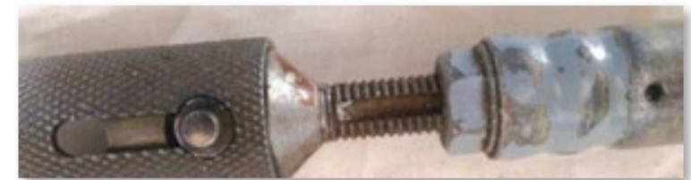
Sleeve fully engaged; locking pin fully out. Note the push rod lock nut is tight/secure and witness hole.
