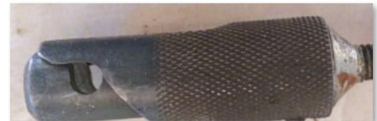
Sleeve locked, pin locked - fully extended
