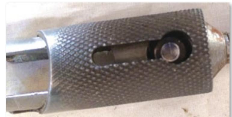
This is the risk: the pin and sleeve are almost correct but the sleeve is a little twisted and the pin is held in.
