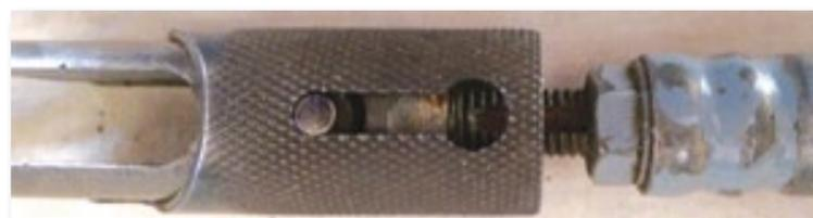
Coupling picture for detail: Sleeve unlocked, pin depressed:
