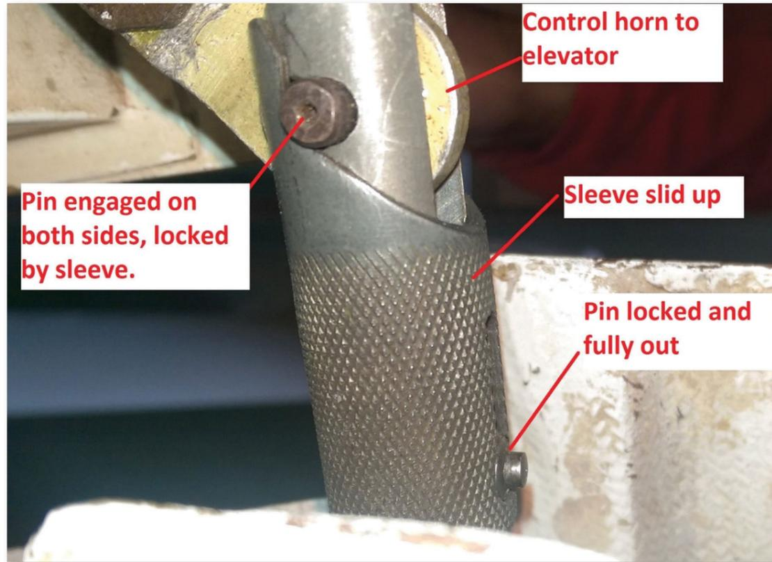
Pin engaged on both sides, locked by sleeve.
