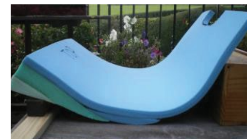
This particular safety cushion insert shows how the energy absorbing foam layers have had to be built up to match the cockpit space available and also to maintain a comfortable body posture for the pilot when seated. In use, the foams are contained within a protective cloth cover.
