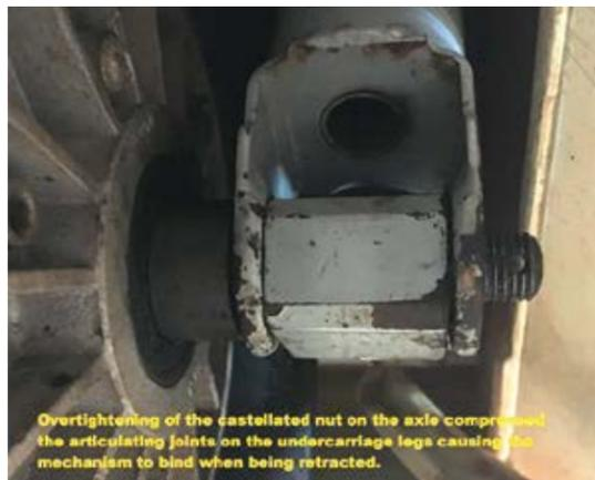
Overtightening of the castellated nut on the axle compressed the articulating joints on the undercarriage legs causing the mechanism to bind when being retracted.
