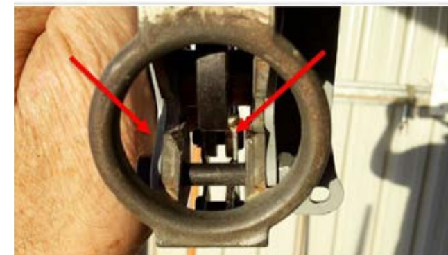
Figure 3: TOST E 22 release. Note the wear on the side plates.
