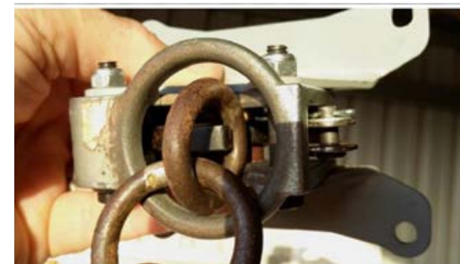
Figure 2: TOST E 22 release. Worn rings wedging under beak.
