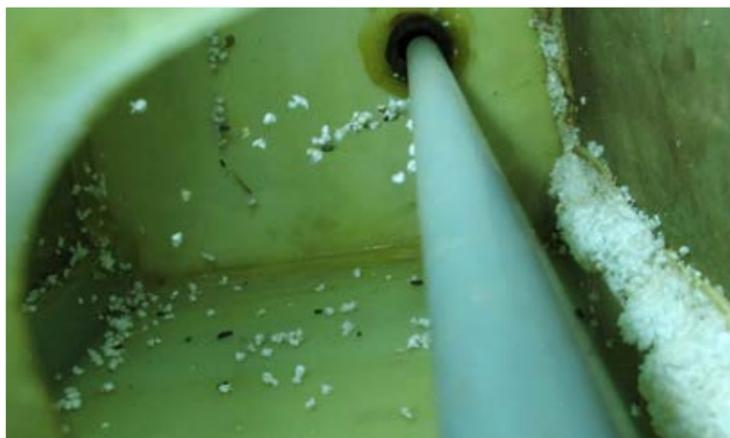
**TOP: 1. Cross bar and support tubing showing surface corrosion.**
