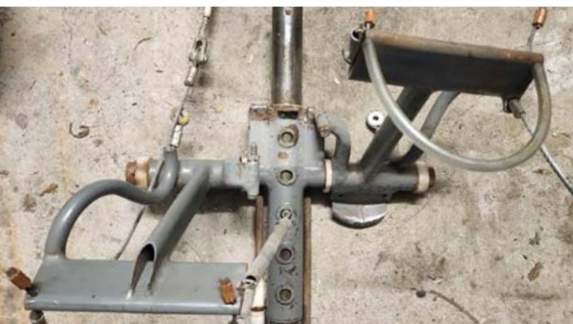
**Figure 2: The pedals had all but seized due to corrosion.**
