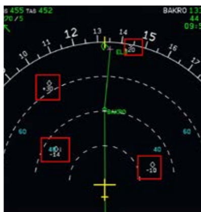
TCAS (traffic collision avoidance systems) are installed in most airlines. However ADS-B, including the Sky Echo, won't reply to TCAS and will not give avoidance advice.
