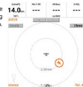
ABOVE: Sky Echo can be displayed on Android phones with XCSOAR and the Traffic app installed.
