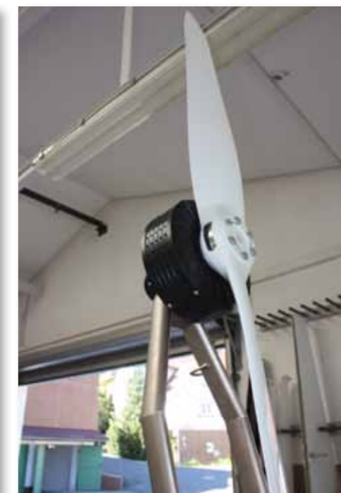
ABOVE: Brushless AC motor with newly developed propeller.
