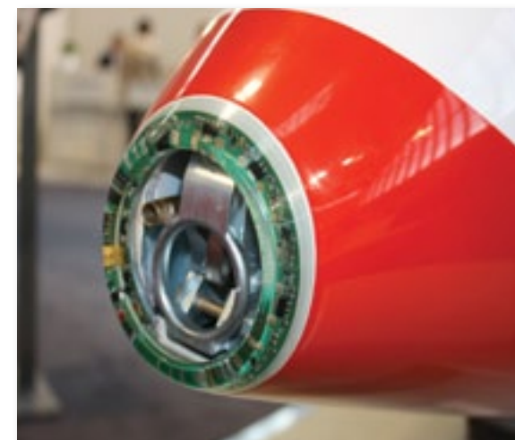
LEFT: DG's new LED flashlight in the nose of a DG 1000 is activated by Flarm to provide an additional warning, especially in head-on situations.
