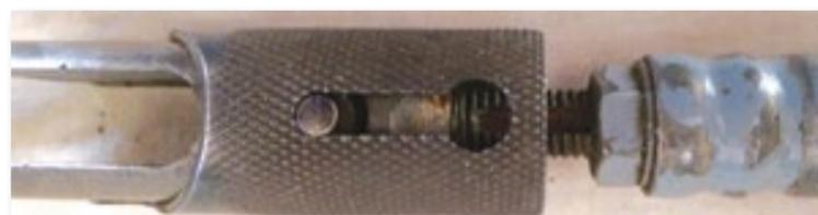
Coupling picture for detail: Sleeve unlocked, pin depressed:
