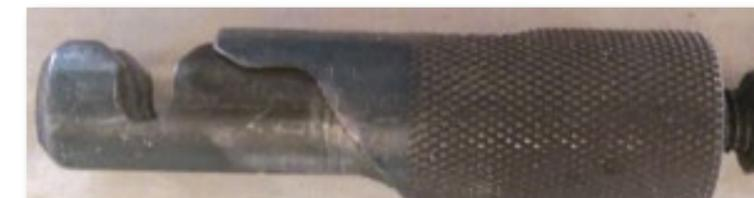
Sleeve and jaws open, ready for assembly. Locking pin just visible but depressed in unlocked position under sleeve
