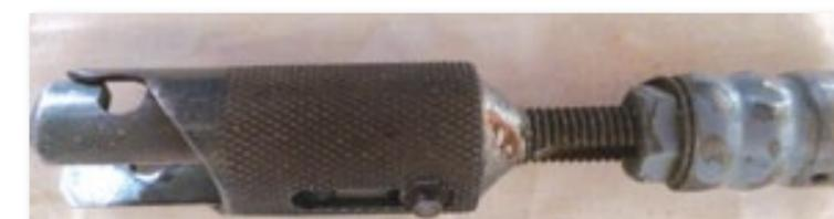
Sleeve locked, pin locked - fully extended
